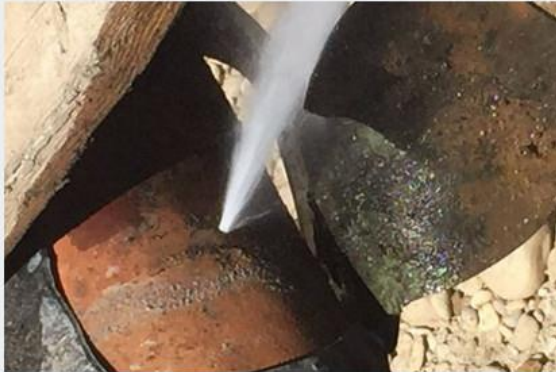
NO Cathodic protection here
